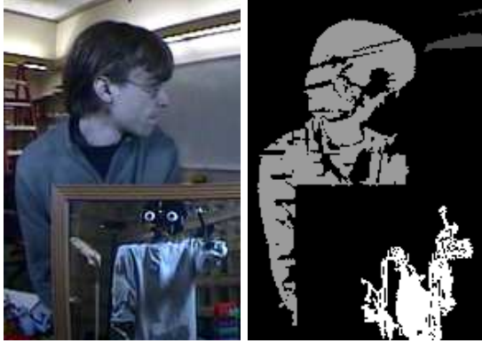
Figure 2: Output from the self/other algorithm while the robot views the experimenter and the robot’s mirror image. The algorithm classifies objects found through background subtraction as “self” (white, bottom), “animate other” (light gray, left), or “inanimate” (dark gray, upper right) in real time.
