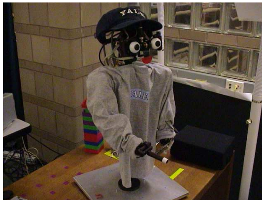
Figure 1: Nico is an upper-torso humanoid robot with the arm and head kinematics of a one-year-old.
