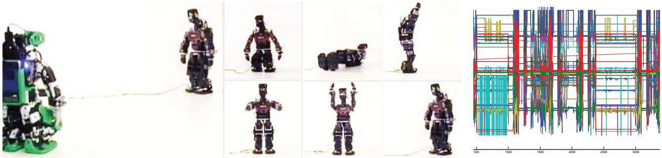
Figure 1: Experiment phase I. Left: A robot performs a series of actions in the world and is observed by the other robot on the left. Middle: Examples of the actions performed by the robot. Right: The resulting raw data stream, containing both the proprioceptive data of the performing robot and the visual features extracted by the observing robot.
