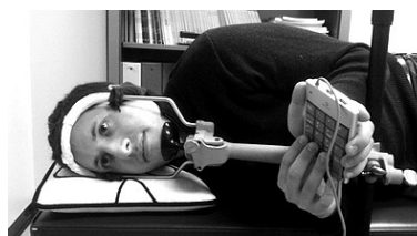
Figure 2: Pole-mounted horizontal chin-rest used in all experiments. Response pad used in Experiment 1.
