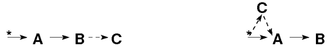
Figure 1: Insertion of C in the queue containing A and B, solid arrows indicate existing links, dashed arrows indicate newly created links. Left: insertion at the end of the queue. Right: insertion at the beginning of the queue.
