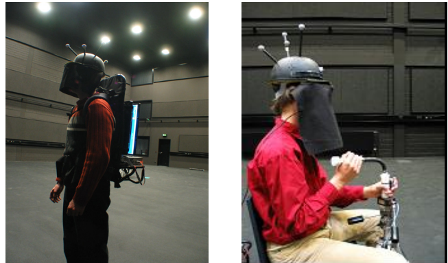
Figure 1: The virtual reality setup. The left image depicts a participant during the learning phase, equipped with a tracking helmet, head-mounted display (HMD), and notebook mounted on a backpack. The right image shows a participant pointing to a target during the testing phase.
